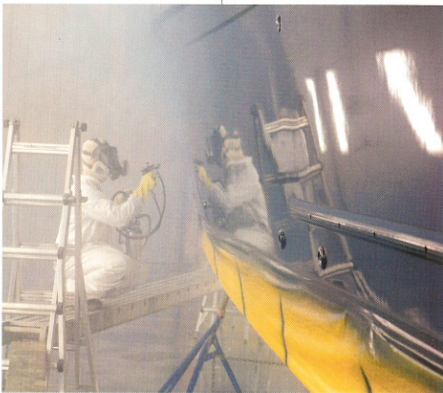
Applying marine-grade paint can be hazardous to your health — it's best to leave this work to professionals with the knowledge and equipment to safely paint your vessel.
