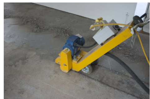
A floor scabblers will quickly remove thick layers of old coatings.
