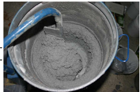
A forced action mixer with a scraper is essential for mixing more than 10 kg batches.
