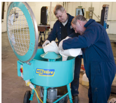
An IMER mixer with bottom discharge is better for larger jobs.
